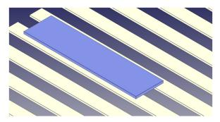
Do NOT place the Adaptive Bed Sensor on only 1 bed slat. Doing so will decrease the performance and lifespan of the sensor.
